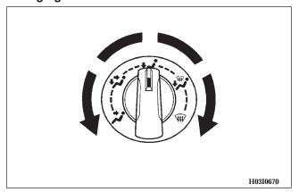
To change air flow to the different outlets, turn the mode selection dial to the desired position.
